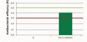
Antibacterial efficacy on S. aureus DSM 346 / E. coli DSM 1576 after a contact time of 24h. K = laboratory internal and not antibacterial control.
