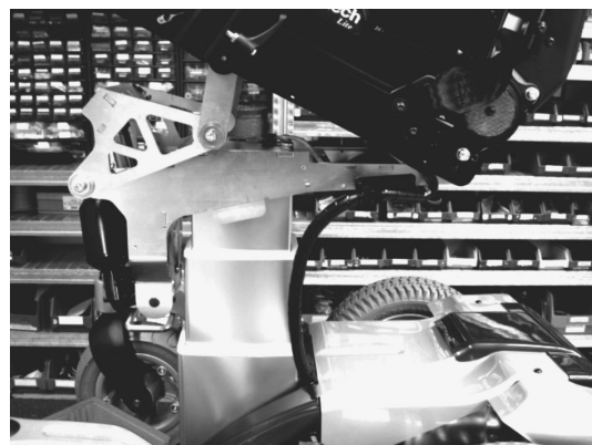
Fig. 6-77 Lifter column completely extended
