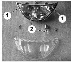
Remove screws (1) on headlight glass.
