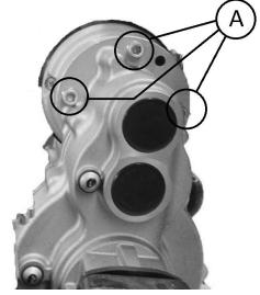
Loosen three Allen screws A.
