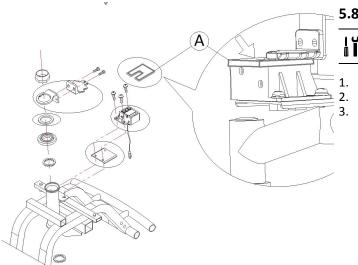
To check position of sensors of curve control device, use measuring gauge B supplied in "Bend speed reducer retrofitting kit".
