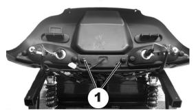
Remove screws (1) on brake light.
