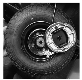
Pull brake out of brake drum.
