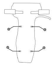
Remove screws (A) on front steering column shroud.
