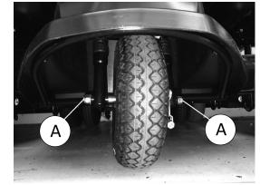
Loosen axle bolts (1) simultaneously on both sides.
