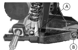
Loosen and remove screw (B) on swing arm. For replacing swing arm, see 5.9.6 Replacing swing arm, page 27.
