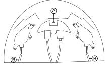
Remove screw (1) or  $\ensuremath{\textcircled{}}$  on headlight under front shroud.
