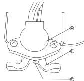
Connect potentiometer (A) and drive lever mounting (B):
