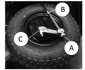
Slacken brake cable using setting screw (A).
