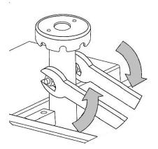
Loosen securing bolt of seat support tube.
