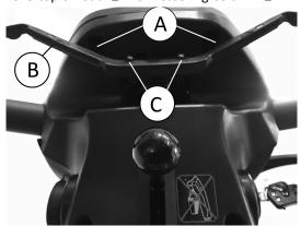
Remove screws (A) below operating console.
