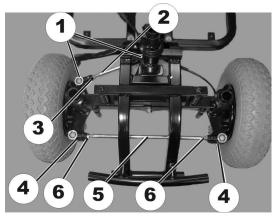
Remove circlip (1) on steering link (2).
