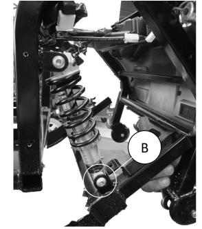
Loosen and remove lower bolt <sup>®</sup> on rear shock absorber on left and right side of the mobility device.
