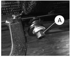
Loosen and remove screw A that attaches swing arm to chassis on left and right side of the mobility device.
