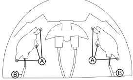
Remove direction indicator screw (A) on chassis.
