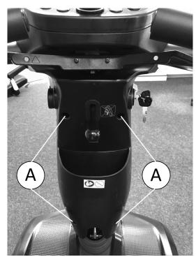
Remove screws (A) on rear steering column shroud.6. Remove steering column shroud.
