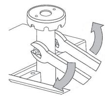
Firmly tighten securing bolt of seat support tube. 14. Reposition seat.
