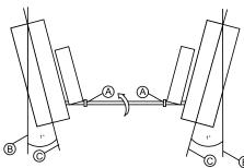
Spin steering link up by 0,5 cm. Wheels stand turned inwards by  $1^{\circ}$   $\bigcirc$  from neutral position B.
