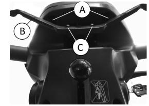
Remove screws (A) below operating console.
