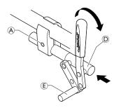
$\bigcirc$   $\rightarrow$  13 Nm / 10 Nm with carbon frame
