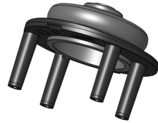
Fig. 6-1 Gaiter Pushed Through The Gaiter Retainer
