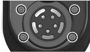
Fig. 4-1 REM050 gaiter retainer screw locations
