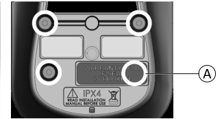
Fig. 4-2 REM060, REM1xx and REM2xx gaiter retainer screw locations. Fourth screw A under label.
